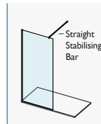
650mm Angled Stabilising Bar included with 450, 500 & 600mm COMPLETE wetroom kits. 1200mm Straight Stabilising Bar included with COMPLETE wetroom kits over 700mm.
