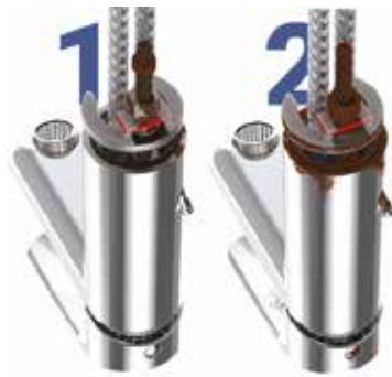
PICTURE 1: Results of the cathodic protection patented by Ramon Soler® after 600 hours salt spray. PICTURE 2: Results without the protection after 600 hours salt spray.
